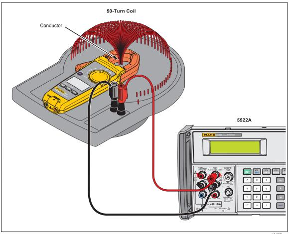
Figure 5. AC Current Test Connections
