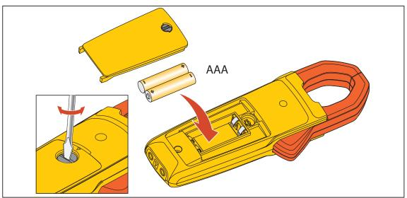
Figure 2. Battery Replacement
