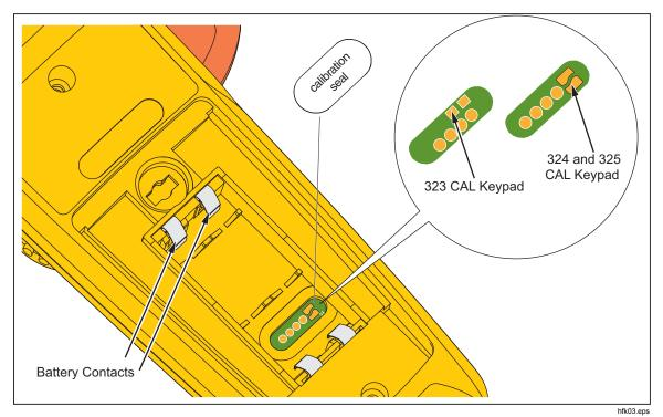
Figure 6. Short the CAL Keypad
