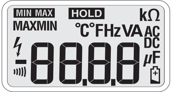
Figure 3. Display Segments (324 and 325 Display is Shown)
